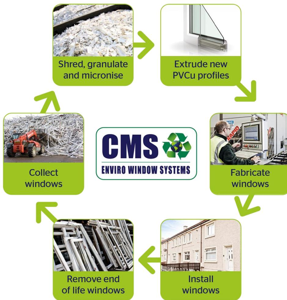
**Figure 1: Recycling process involving u-PVC in Windows**
