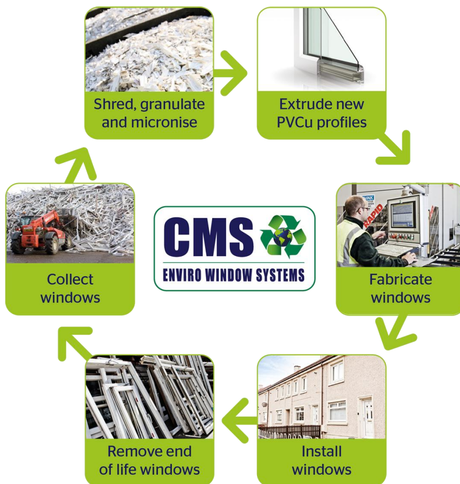
Figure 1: Recycling process involving u-PVC in Windows
