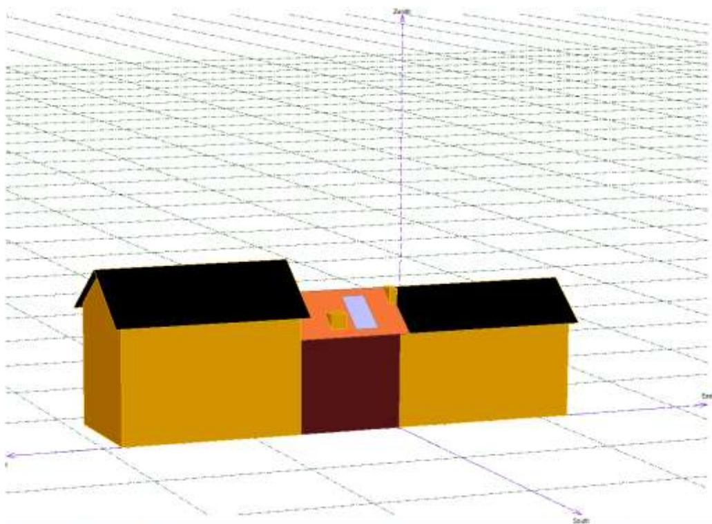
Fig. 18 Image showing solar shading analysis produced by solar PV software
