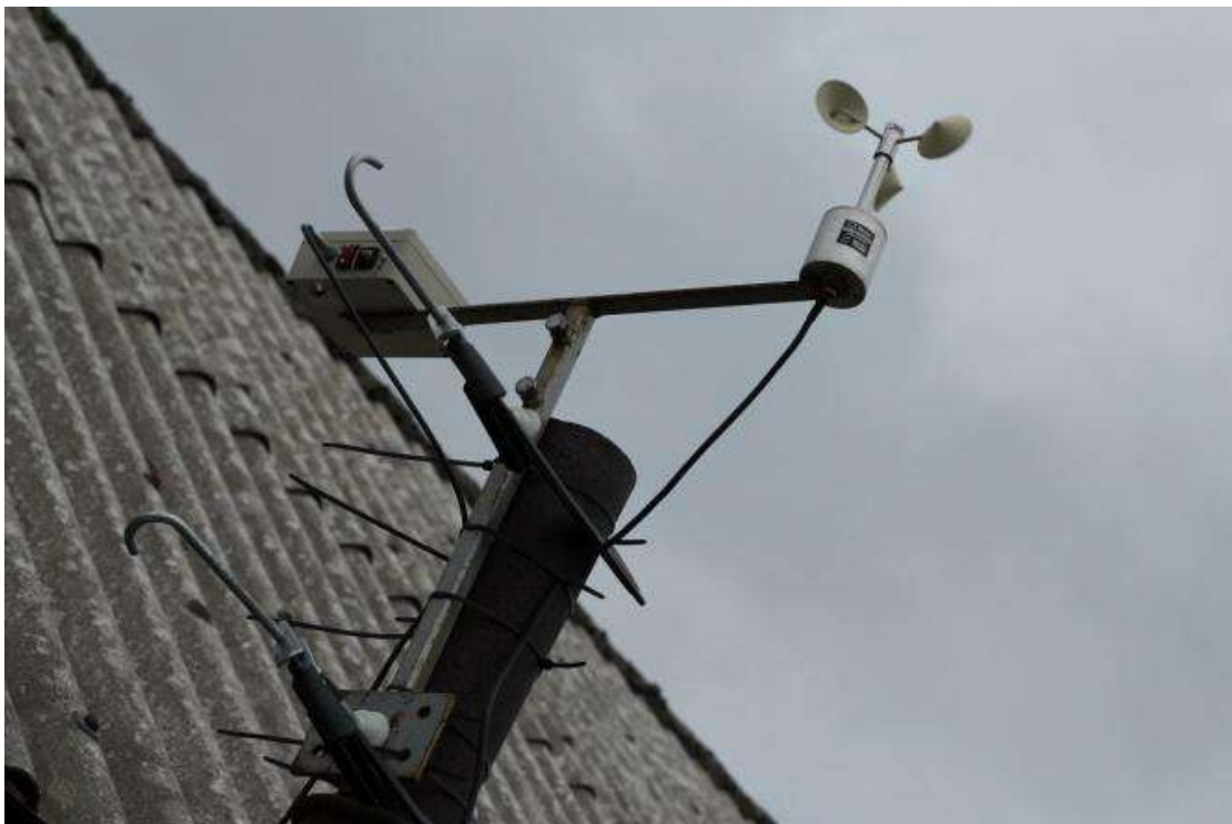
Figure 5. Horizontal solarimeter and anemometer (Photograph from Uist HtT Housing Project 2011-12 Final Report Part 2).
