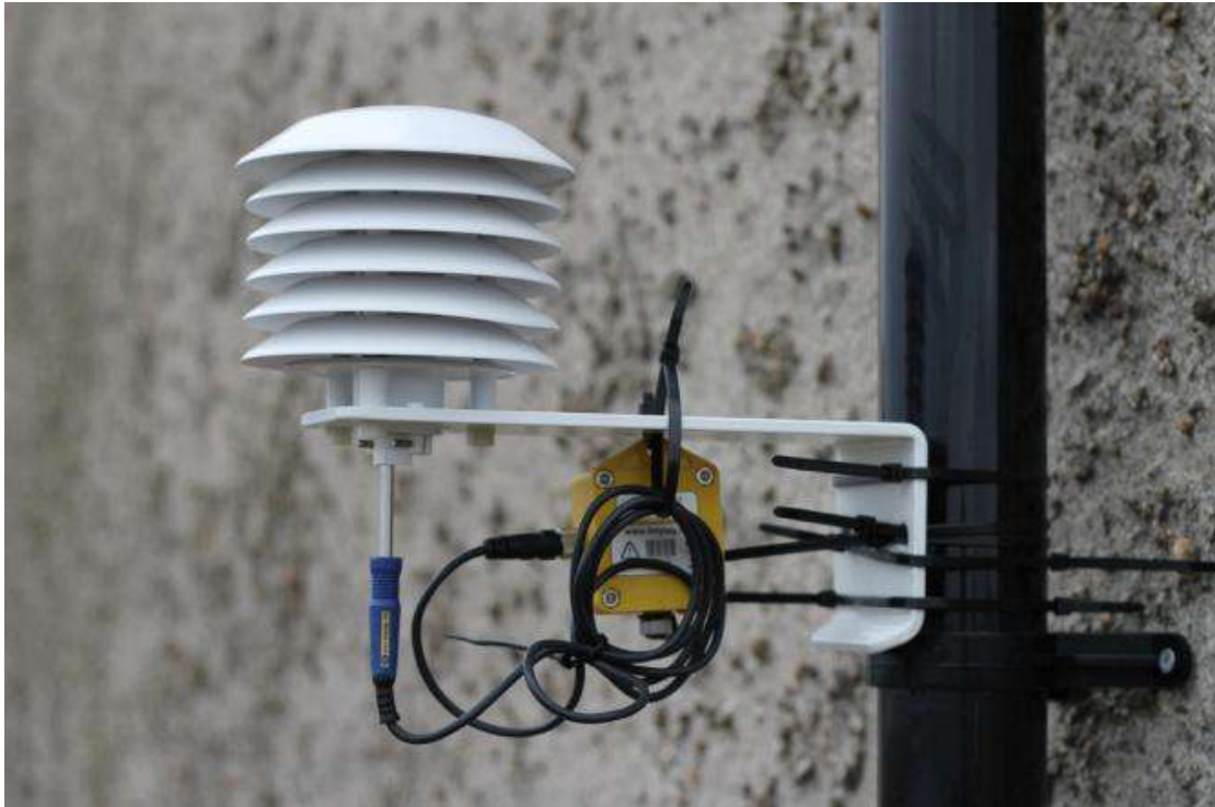
Figure 4. External Tinytag air temperature sensor with shield (Photograph from Uist HtT Housing Project 2011-12 Final Report Part 2).
