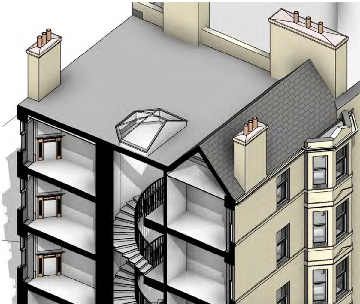
A Late Victorian Edinburgh Tenement, showing the arrangement of pitched and flat roofs. Grigor Mitchell Architect Ltd.
