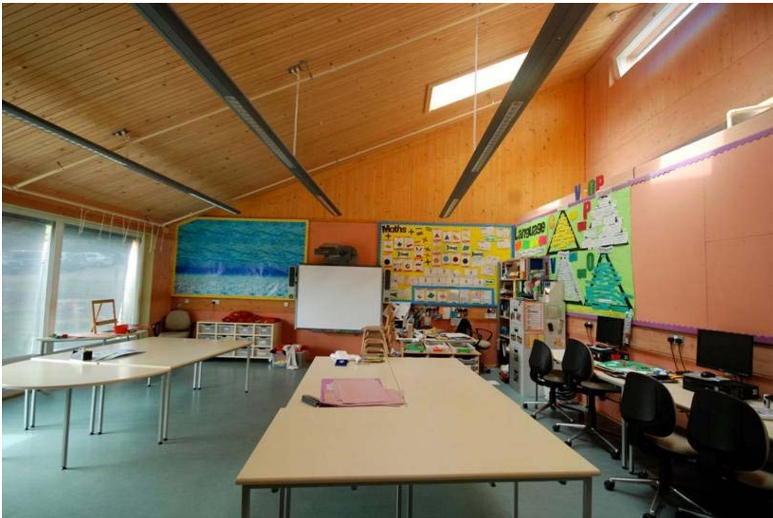
Figure 10. Acharacle school has natural ventilation with external shading screens when very bright, still giving good daylight in the room and allowing lights to be off
