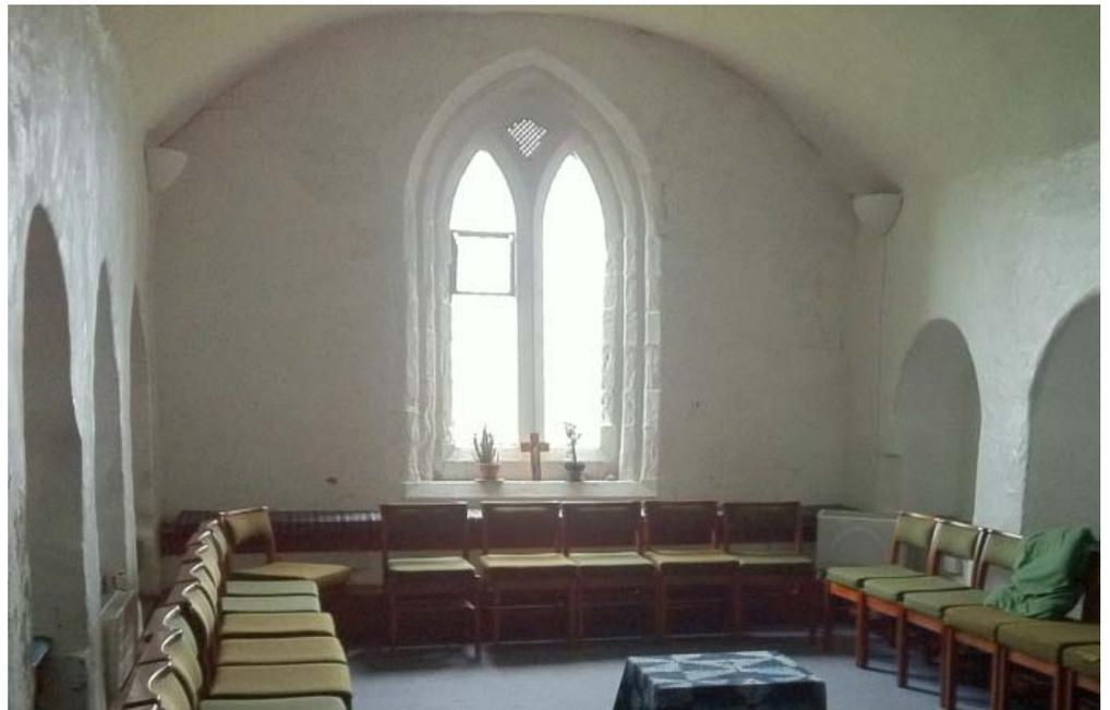
Figure 2. Splayed window reveals, white mullions, astragals and light ceilings and walls reduce glare, making the most of the daylight
