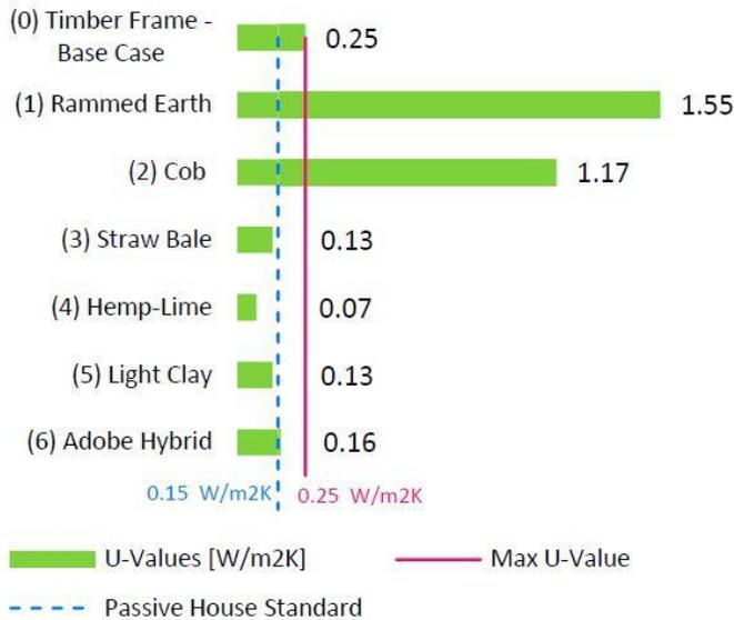
Figure 3. Thermal Transmittance (U-Value)
