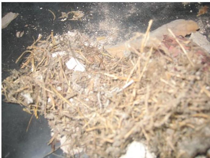
Picture 5. Sample of debris removed from the wall during the trial despite the cleaning prior to the start
