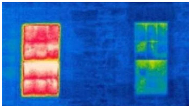
Fig. 2 Thermal image showing the reduction in heat loss with shutter closed (left) and shutter open (right)
