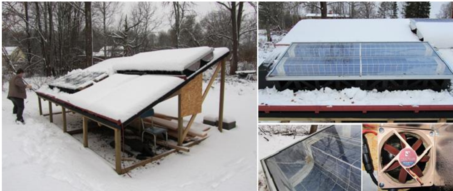
Figure 4: PV/T HR Roof Integrated System Mock-up Built by Finsun Inresol in Alvkarleby, Sweden
